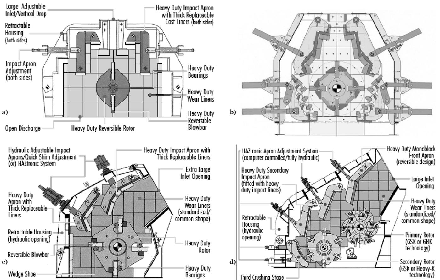
Fig. 1. Examples of impact crushers design [6]
