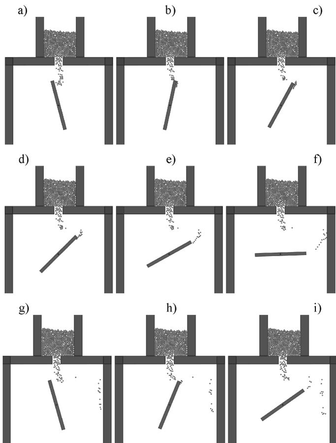
Fig. 3. Flow of crushed material in the impact crusher
