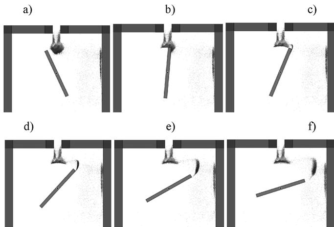
Fig. 2. Stages of forming stream of particles, due to impact of blow bar
