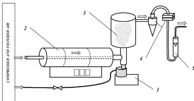
Fig. 1. Scheme of the experimental set-up: 1 – ultrasonic nebulizer, 2 – tubular furnace (heater), 3 – expansion chamber, 4 – fibrous filter, 5 – flowmeter
