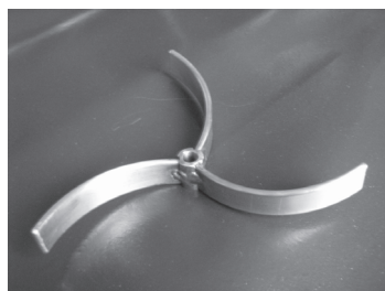
Fig. 1. Experimental layout with curved blade turbine
