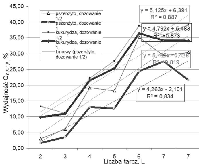
Fig. 1. Percentage values of target mass efficiency  $Q_{0.8+1.6}$  for a variable number of discs and a variable method of biomaterial feeding (in relation to the general mass efficiency)
