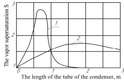
Fig. 2. Supersaturation along the length of the condenser pipes at various temperatures cooling water: 1 – 293 K, 2 – 313 K
