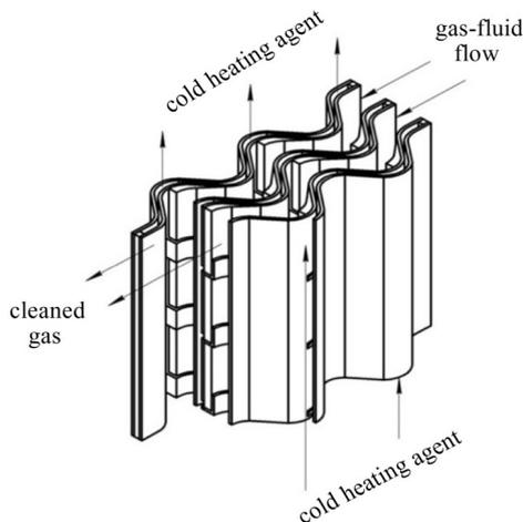
Fig. 1 Scheme of the flows moving during the inertial filtering process by condensation [Sklabinsky et al., 2014]
